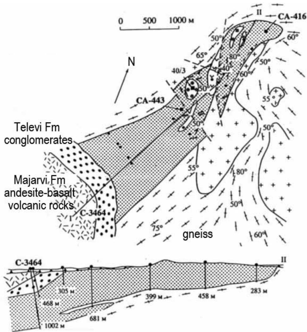
Fig. 13. Scheme of the geological structure of the layered intrusion Mt. Generalskaya.
