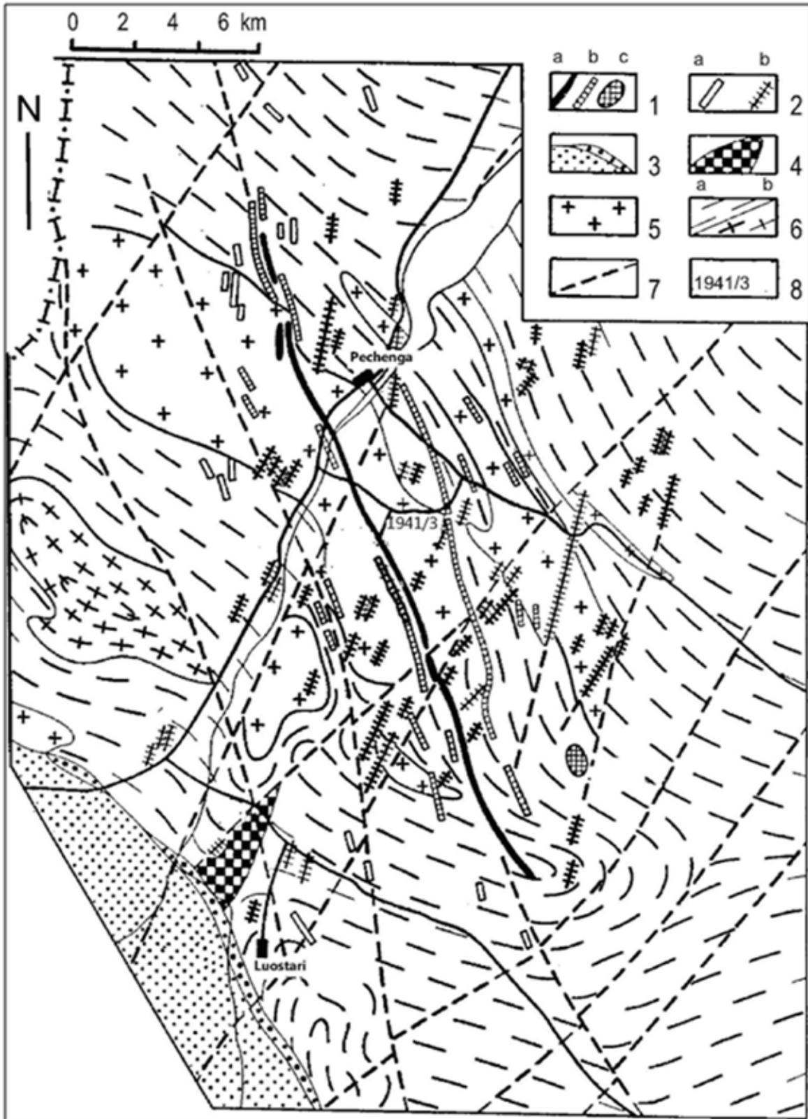
Fig. 2. Geological sketch map of the Nyasyukka dyke complex. 1 – the Nyasyukka dyke complex: a – peridotite, b – olivine gabbro, c – olivine pyroxenite; 2 – Palaeoproterozoic dykes: a – dolerite, b – quartz dolerite; 3 – basal conglomerate and volcanic rocks of the Pechenga Complex; 4 – Mt. Generalskaya mafic layered intrusion; 5 – Archaean plagio-microcline granite; 6 – Archaean amphibolite, gneiss, high-Al schist; 7 – fault; 8 – U-Pb age.
